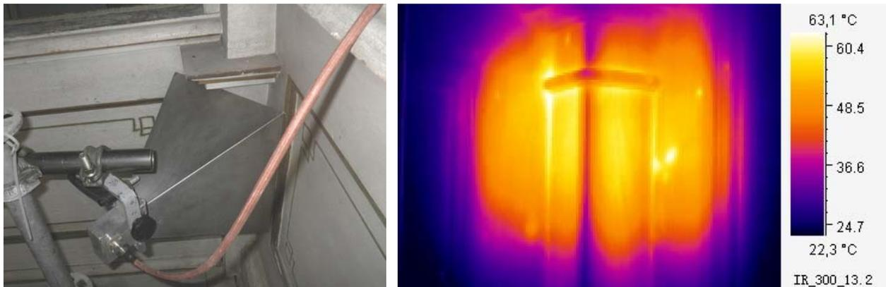
**Figure 2: Treatment of a gallery balustrade with a coloured surface, infested with the ordinary furniture beetle (*Anobium punctatum*), an infrared recording taken shortly after the removal of the antenna.**
